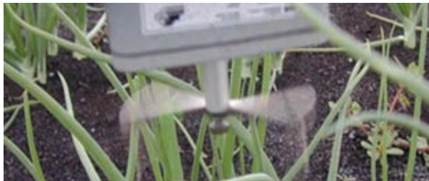
Figure 11. A typical rotating-arm spore sampler used to monitor B. squamosa spores in the field.
